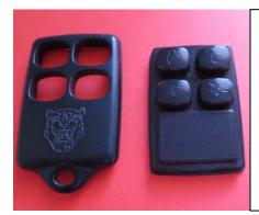
Next place top part of plastic shell over key pad making sure buttons fit in respective holes.
