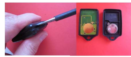
Use small flat screw-driver to open remote key on the split line to separate it into two parts.
