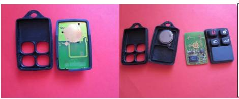
Next you will be separating key button pad containing electronic board from plastic shell.
